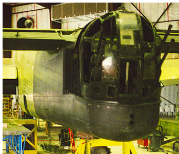
Boulton Paul Tail turret of the Halifax armed with four Browning .303 machine guns.
