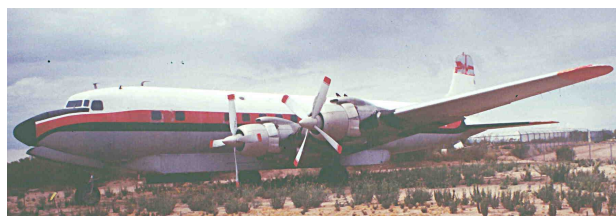
A DC-7, converted to fire bombing. Note the tank under the fuselage.
