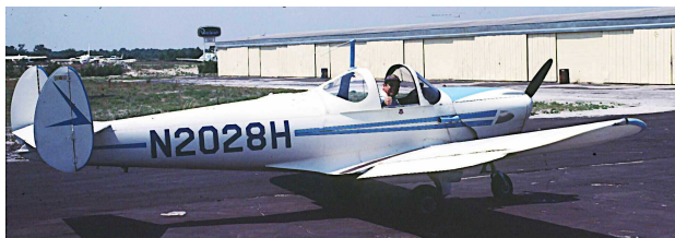
Maj Rocketto in an Ercoupe 415-C on a ferry flight to Florida. The aircraft has no rudder pedals.
