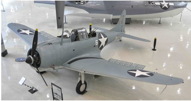
Douglas SBD-2 Dauntless, an actual veteran of the Battle of Midway displays its unique dive brakes at the USN Museum at Pensacola. Jerry Coleman flew one of these during the Guadalcanal campaign.
